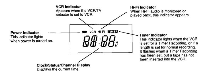
Briefly displays VCR status when function button is pressed. Also, briefly displays the channel number selected, "L1" or "L2"
