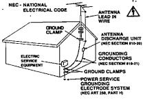
**INSURE SAFE ANTENNA** AND CABLE CONNECTIONS If an outside antenna or cable system is connected to the equipment, be sure the ANTENNA equipment, be sure the DISCHARGE UNIT antenna or cable system is (MEC SECTION 810-20) grounded so as to provide grounded so as to provide some protection against built up static charges and voltage surges. Part 1 of the Canadian Electrical Code, in USA Section 810 of the National Electrical Code, ANSI/NFPA
