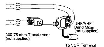
If your TV has both post and screw-type VHF terminals, using the post connection is recommended to minimize signal loss.
